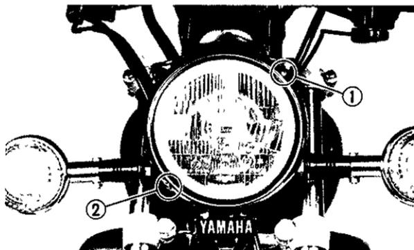
1 Horizontal adjusting screw 2 Vertical adjusting screw
