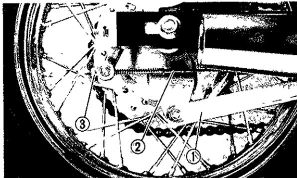
1 Tension bar    2 Brake rod    3 Adjuster
